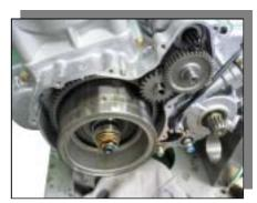
• Remove Oil Filter Cover and take out Oil Filter CP, O-ring and Spring (Filter).
