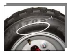
Position the wheel so that the air valve [A] is toward the outside of the vehicle.
