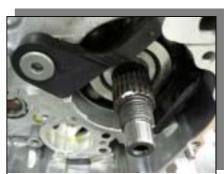
• Put Timing Chain from the Cylinder Head side and set in position as shown in Attachment (2).
