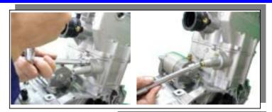
Adjust valve clearance with thickness gauge adopted at TDC position in the following procedures;
