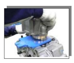
• Install Chain Guide 1 onto Cylinder.
