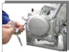
• Tighten Filter Cover plug to the specified tightening torque.
