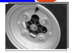
Remove the caliper by taking off the mounting bolts, and let the caliper hang free.
